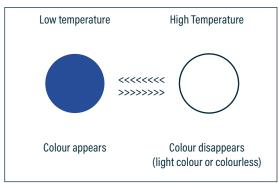
The color change temperature range covered by the thermochromic pigments is 5°C to 60°C.
