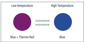
By mixing different thermochromic inks with different temperature ranges, it is possible to get an ink with three shade moves.
